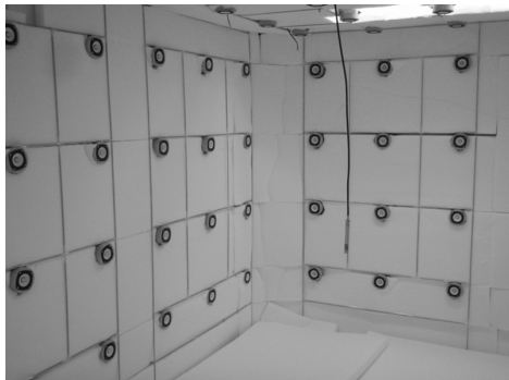
Figure 5: Appearance of the surroundng loudspeaker array after installing the absorption materials
